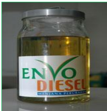
Palm Methyl Ester 100% concentration before blended with diesel and sold at petrol stations in Malaysia (left). Palm oil fresh fruit bunch, source of crude palm oil used to produce palm methyl ester (biodiesel) (right).
